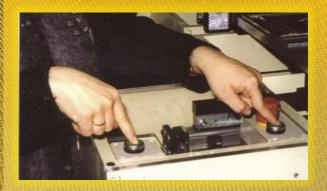
• The machines Pallet system allows for part handling without the need for the operator to handle fabrics in the hot areas of the machine
